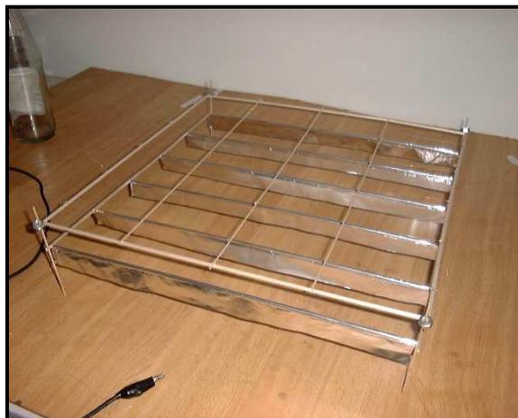
Lifter designed with parallel corona wires spaced at 1.3d
