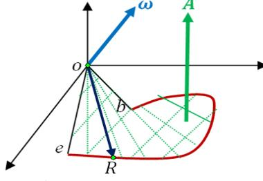
Figure 4.  $\Delta t = (4\gamma/c^2)\omega \cdot \mathbf{A}$  where  $A$  is the area subtended by the circuit and the lines connecting its ends  $e$  and  $b$  with the center of rotation.
