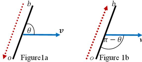
In both figures the rod  $ob$  is translating in  $S$  at a constant velocity  $\mathbf{v}$ . The red arrow points in the direction of a light pulse that starts from one end (an emitter) and ends at the other (receiver). The angle between the radius vector of the emitter relative to the receiver and the velocity  $\mathbf{v}$  is  $\theta$  in Fig. 1a and  $\pi - \theta$  in Fig.1b.
