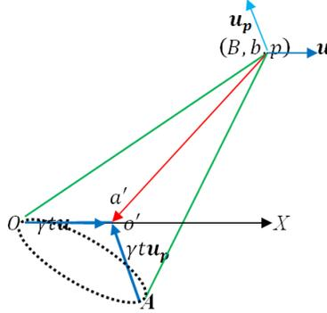
Fig. 5. Pulses from sources at  $B$  that have velocities resulting from rotating the velocity  $u$  of the source  $b$  about  $Bo'$  take the same time to arrive at  $o'$ .
