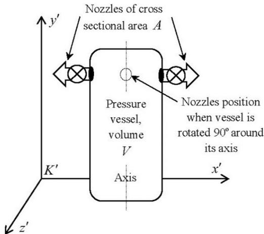
Fig. 1 Experimental arrangement
