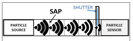
Figure 16. Proposed Experimental Design. Small aperture plates (SAP) inserted at regular intervals to reduce the number of particles or portion of the wave advancing to the sensor. This shutter at the exit of the last SAP is set to close for intervals shorter than time T, T being the shortest interval detected between the arrival of any two particles during the initial particle count run, with the shutter wide open.
