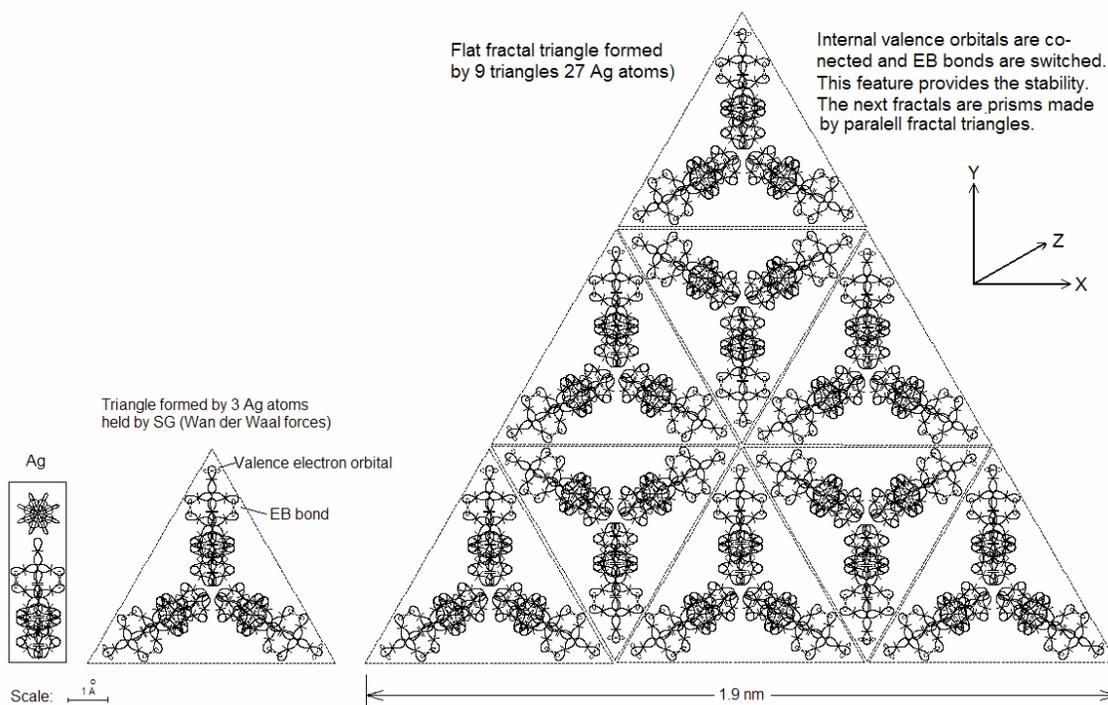
**Fig. 18.** One side of silver nanostructures, shown as a sheet, illustrated with the BSM-SG atomic models. The left sheet is formed of 3 silver atoms, while the right sheet is formed of 27 silver atoms. The fractal build-up allows obtaining triangular sheets with different sizes in the nanoscale range.
