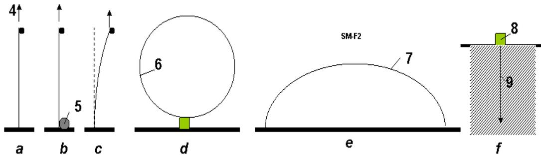
Fig. 9. Some construction from AB-string. *Notations:* *a* – vertical string (AB-needle). The big lift (support) force 4 does not depend from length; *b* – lifting the load to any altitude. 5 - spool of AB-string; *c* – stability of AB-string; *d* – ring 6 from AB-string; *e* – bridge (long arm) from AB-string; *f* – research of the Earth crust interior: 8 - installation (spool of AB-needle), 9 – AB-needle (string, cable).
