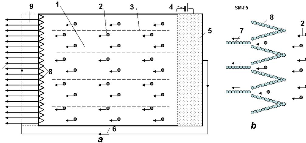
Fig. 13. Method particle traps for production of the AB-needles. *Notations:* a – device; b – particle traps; 1 - vacuum cell; 2- charged particles; 3 – magnetic lines; 4 – electric issue for the acceleration nets; 5 - plasma from particles; 6 – flow of electrons; 7 – AB-needles; 8 – trap made from AB-matter for the charged particles ( $p$ ,  ${}^2\text{H}$ ,  ${}^4\text{He}$ , etc.); 9 – cell for cover the AB-needles by electrons.
