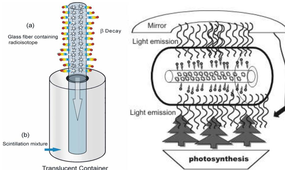
**Fig1. Radioisotope excited scintillation lamps.** a) Glass fiber chip of encased radioactive isotope and scintillation mixture showing Beta Decay, with atomic disintegration and emitting  $\beta$  particles. b) Being introduced into a translucent cylinder made of additional layers of scintillation substances, like sodium iodine (NaI), after excited molecules return to ground state emit scintillation light and glows like a lamp.
