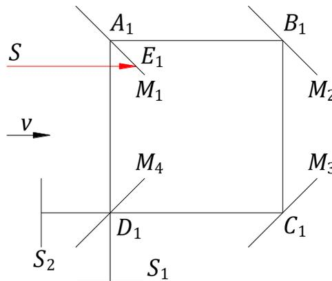
**Figure 7.** Interferometer at the initial instance.
