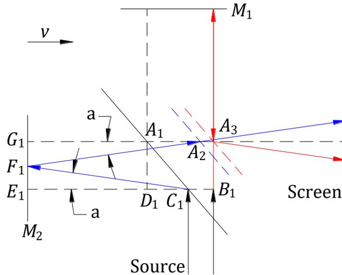
**Figure 4.** Light paths geometry when the interferometer is rotated by  $270^\circ$  from its initial position.
