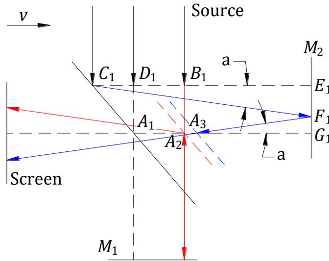
**Figure 2.** Light paths geometry when the interferometer is rotated by 90° from its initial position.
