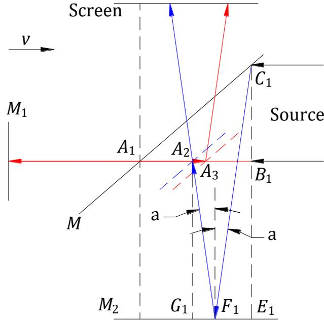
**Figure 3.** Light paths geometry when the interferometer is rotated by 180° from its initial position.
