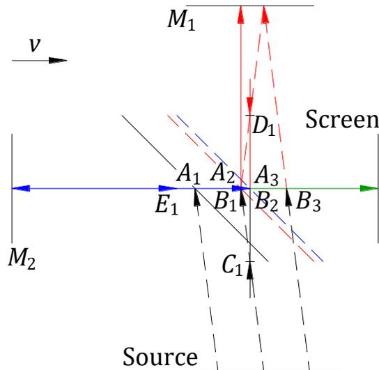
Figure 4. Derivation of the light paths when the interferometer is rotated by  $270^\circ$  from its initial position.
