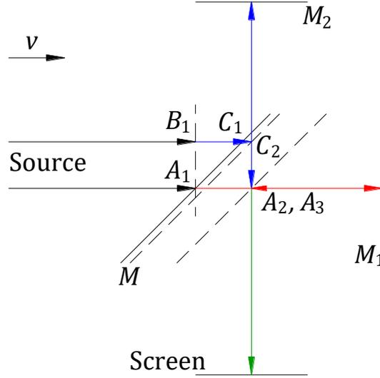
Figure 1. Derivation of the light paths with the initial position of the interferometer.
