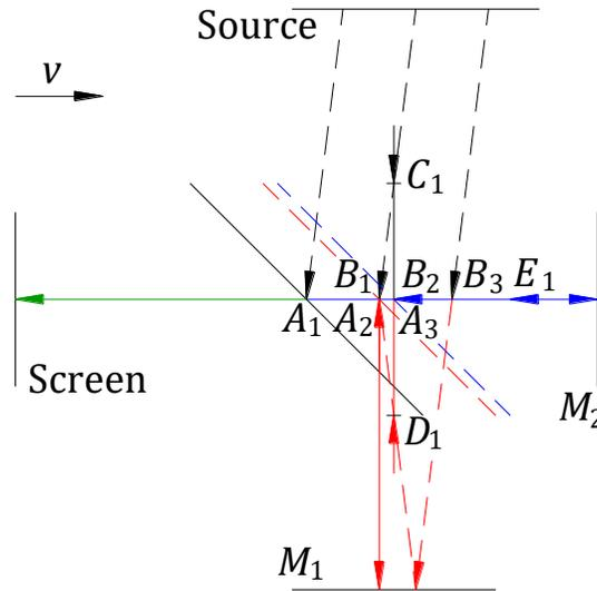
Figure 2. Derivation of the light paths when the interferometer is rotated by 90° from its initial position.
