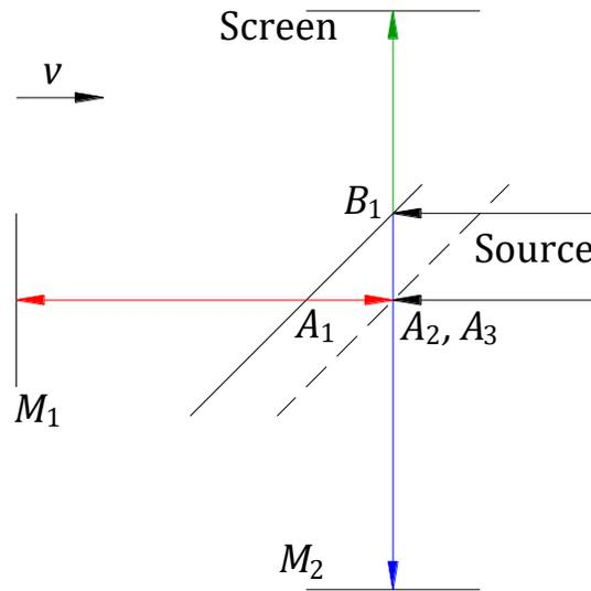
Figure 3. Derivation of the light paths when the interferometer is rotated by  $180^\circ$  from its initial position.
