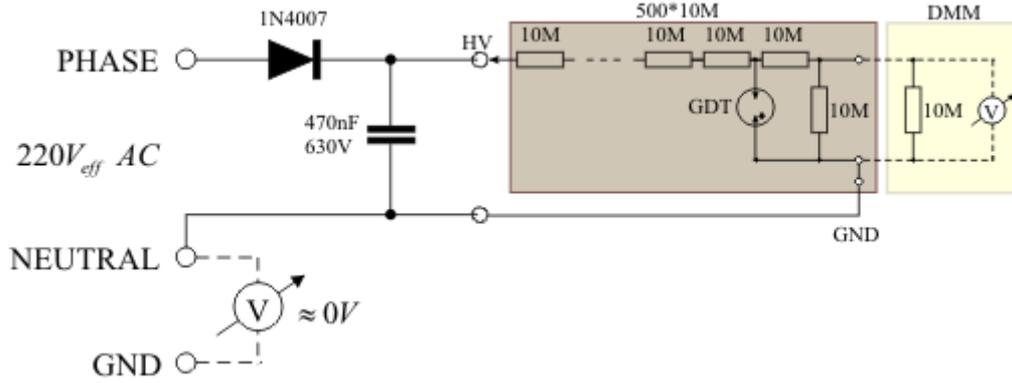
Figure 22: DC Calibration circuit of the HV probe.
