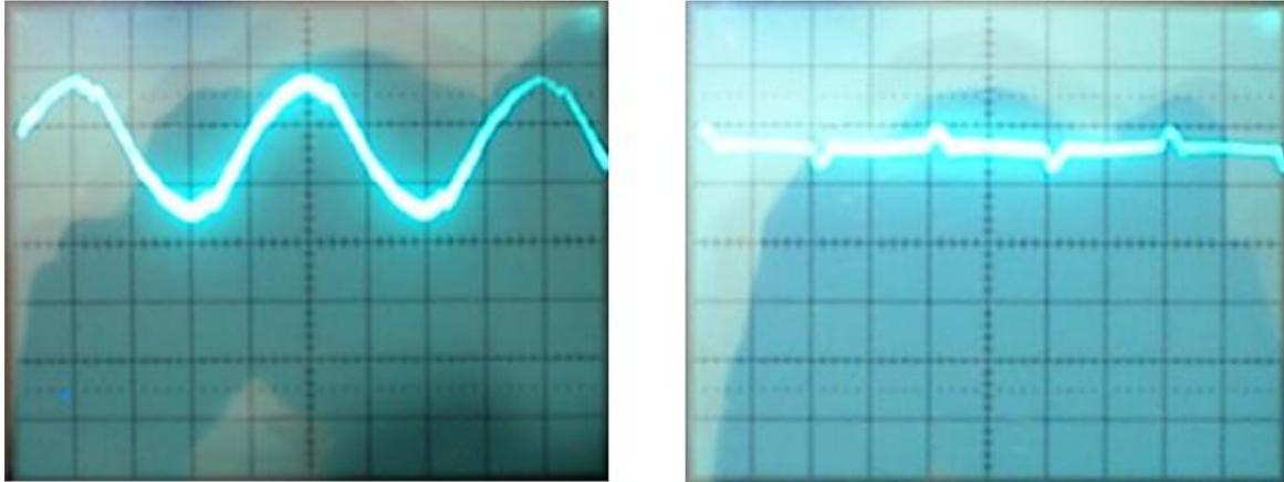
Figure 28: The unfiltered and the filtered output signal shapes of the probe when measuring the 320 V DC on the rectifier (0.2 V/div; 5 ms/div).
