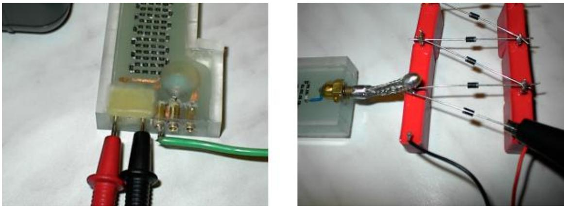
Figure 29: The standard DMM probe tips tightly fit in the connectors, and the elastic HV probe tip touching the test point on the rectifier.
