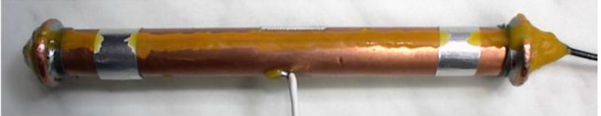
Figure 10: The assembled capacitor sealed with bee's wax, ready to be filled with paraffin oil.
