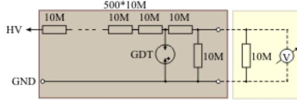
Figure 19: HV probe circuit diagram.
