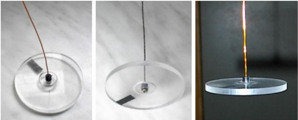
Figure 13: The acrylic disc fixed to the bottom end of the torsion pendulum wire and hanged from the ceiling.
