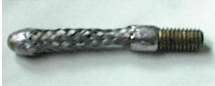
Figure 23: The flexible HV probe tip.
