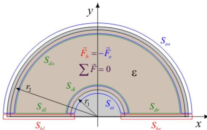
Figure 6: Sub volumes for surface force density integration (thickness exaggerated).
