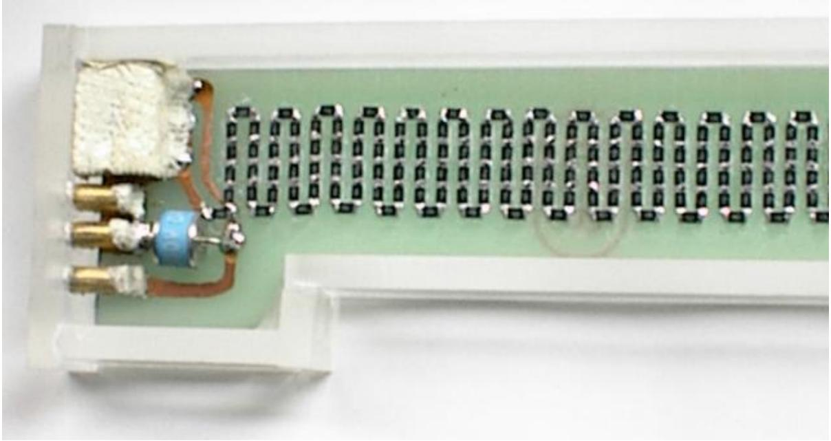
Figure 25: The PCB within the acrylic pot with sealed connector openings.
