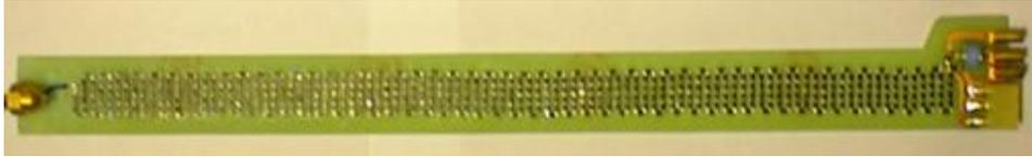
Figure 21: The PCB with mounted parts and soldered resistor-chain.
