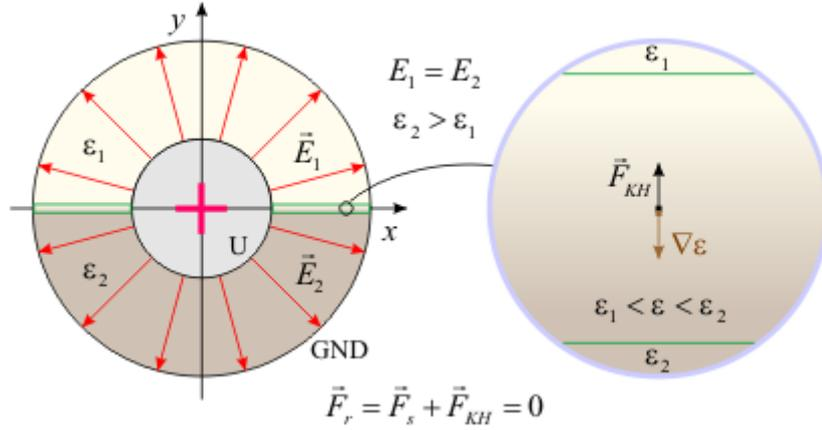
Figure 7: Boundary layer of finite thickness between the two dielectrics.
