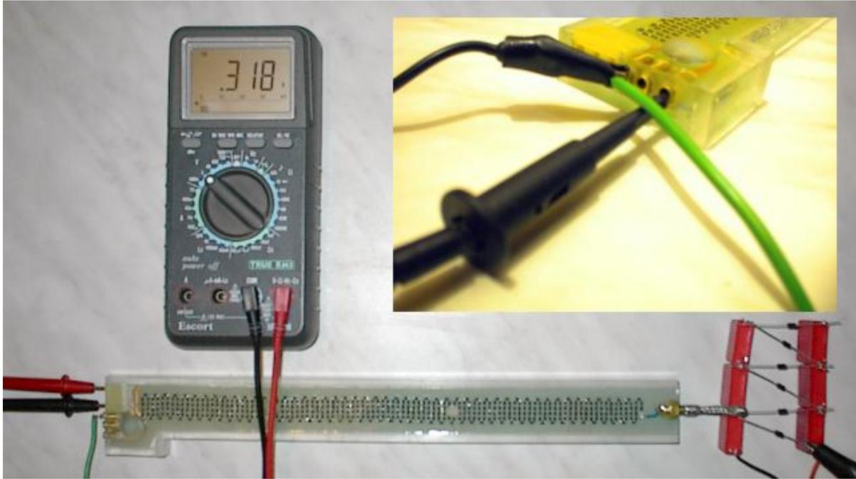
Figure 26: Checking the transfer ratio of the probe (0.318 V is indicated), and an illustration of the oscilloscope's probe being hooked onto the output connector through the screw-holes at the bottom.
