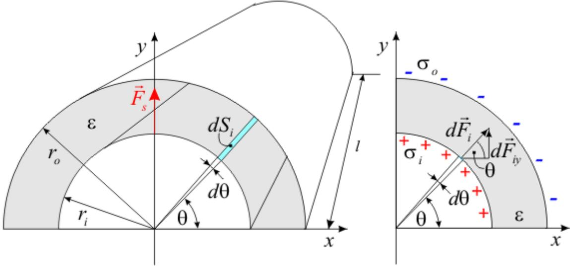
Figure 2: Calculating the  $y$  component of electrostatic pressure forces in the top  $180^\circ$  sector.
