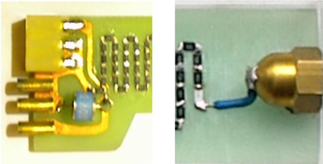
Figure 24: The output connectors and the tip holder brass nut.
