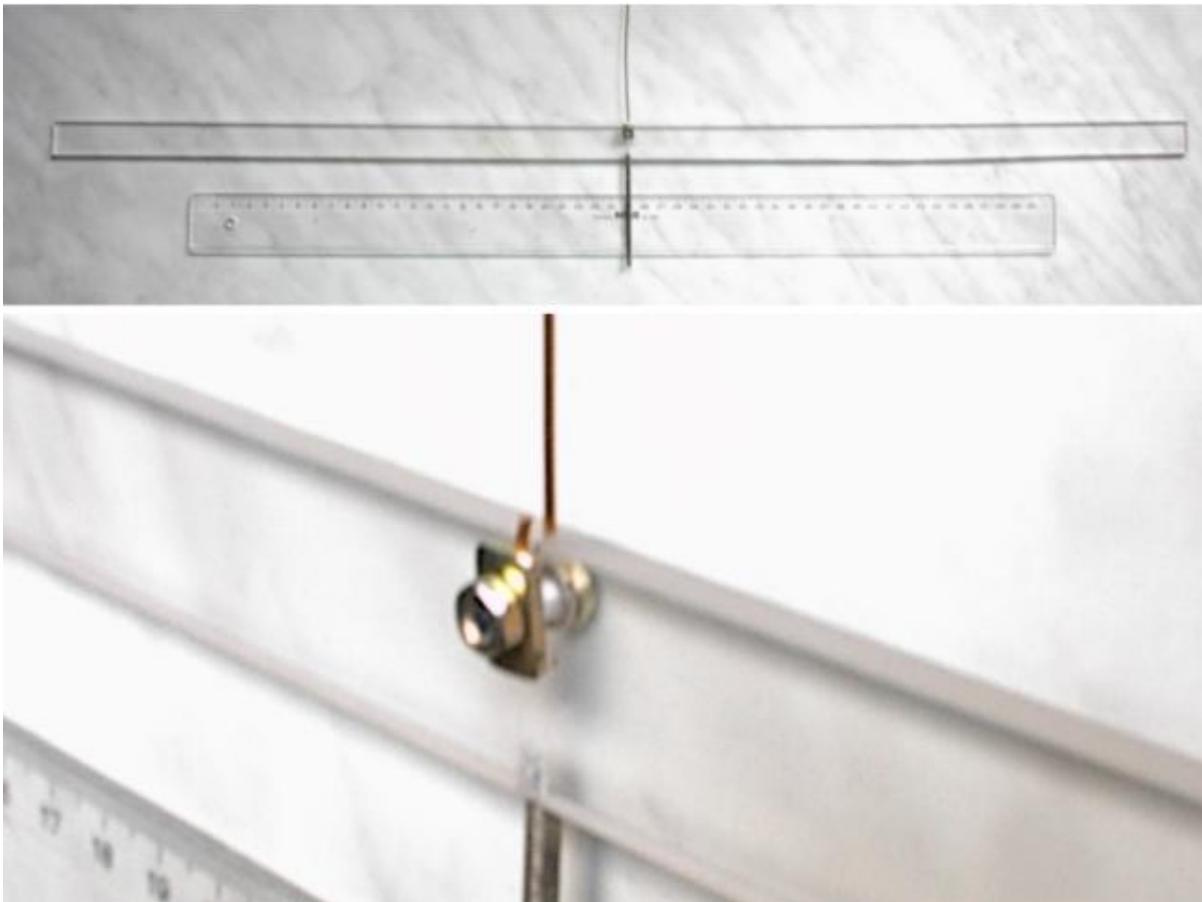
Figure 14: The acrylic beam with the stabilizer shaft attached to the torsion pendulum wire.
