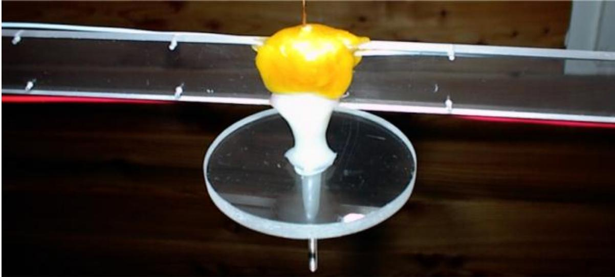
Figure 17: The HV insulation to prevent sparking between the HV shaft and the GND wire.
