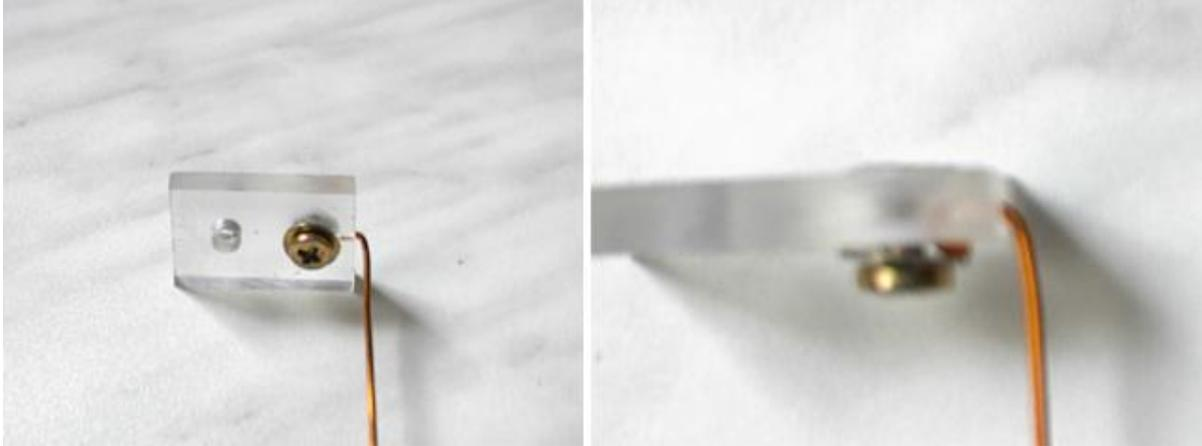
Figure 12: The upper end of the torsion pendulum wire embedded into a holder acrylic block using a bolt & nut (the nut at the top is melted into the plastic and not visible).
