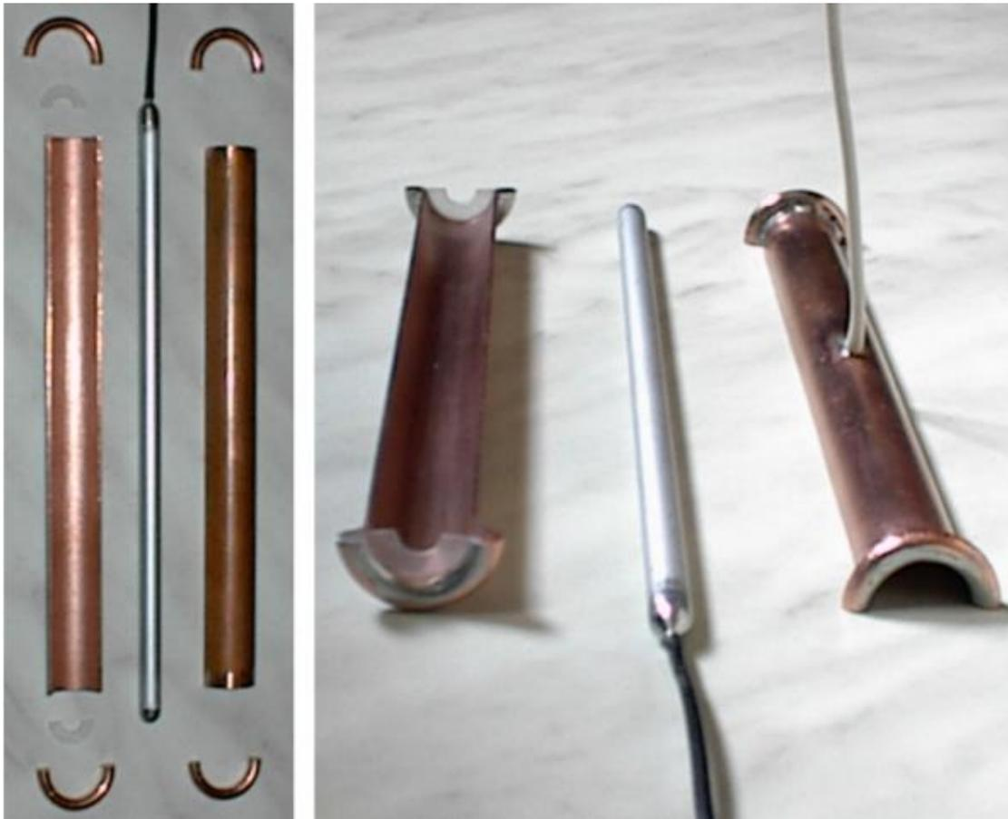
Figure 8: Parts of the coaxial cylindrical capacitor with two different dielectric sectors.
