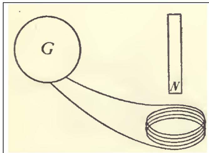
Observation TWO Moving the magnet *faster* increases the intensity of the induced electric current.
