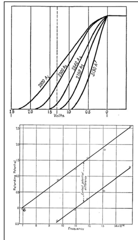
Observe that to every wavelength (frequency) there is a retarding voltage for which the photoelectric current becomes zero – this is the stopping voltage  $V_{stopping}$  which, when plotted against frequency, gives a straight line. The gradient of this line can be found from the graph and comes out equal to the ratio  $h/e$  (the ratio of Planck’s constant  $h$  to the charge of the electron  $e$ ):
