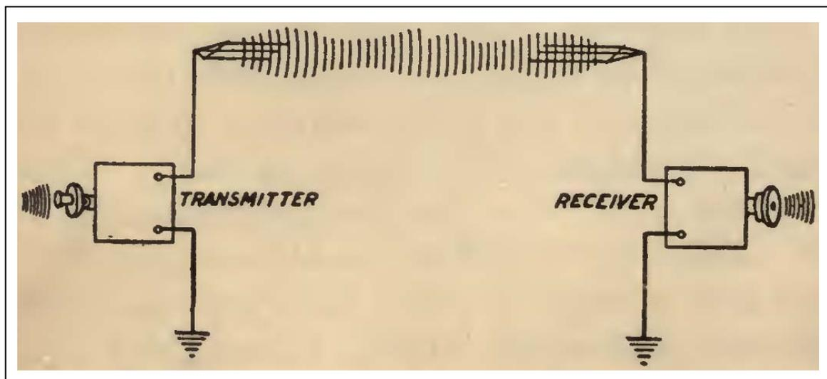
We have shown in Part II that the radio waves produced by the electric currents oscillating in the transmitting antenna are waves in the aether, magnetic in nature. The electric currents that these magnetic waves produce in the receiving antenna are due to the phenomenon of electromagnetic induction.
