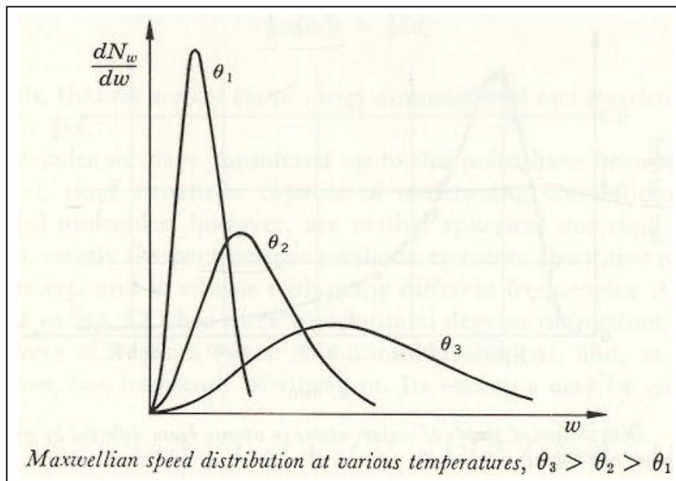
Observe that at higher temperatures there are, on the whole, more particles with great velocities than at low temperatures.
