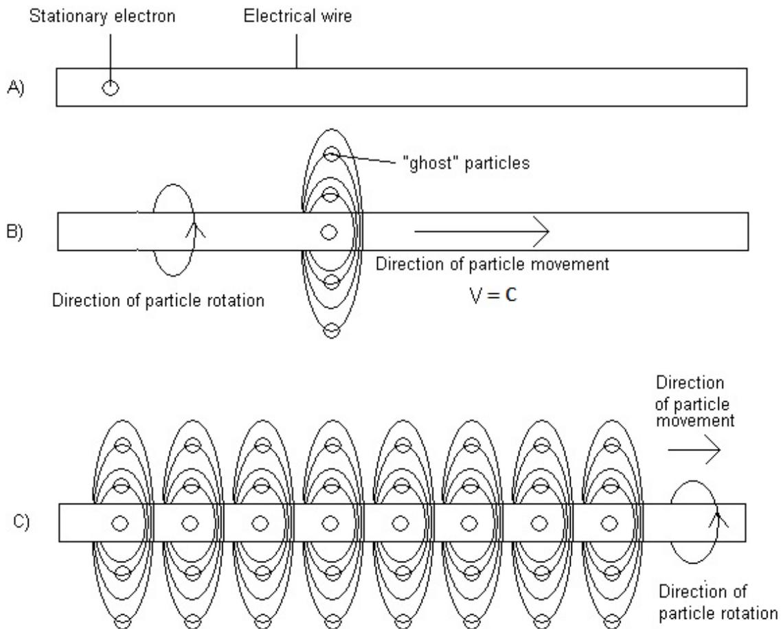
**Figure 5:** In A), we see a stationary electron in a wire. If this electron moves through the wire at speeds far below  $c$ , then the particle simply moves in a straight line through the wire, and no magnetic field is observed.
