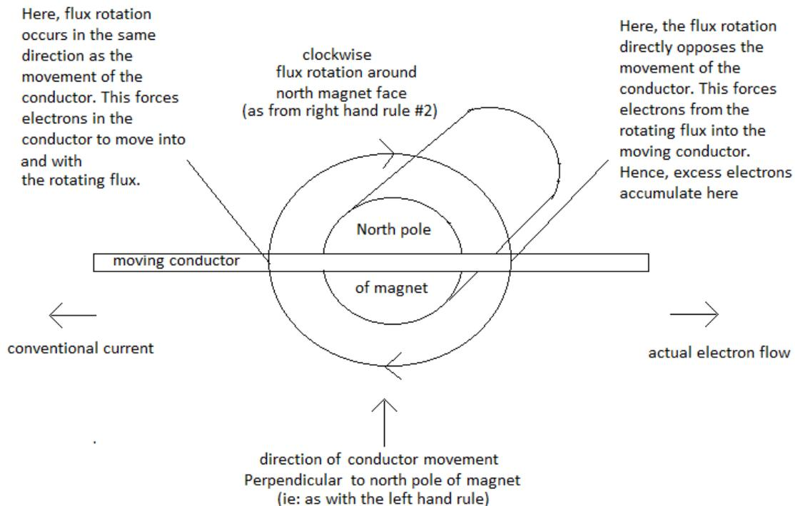
**Figure 9, how induction occurs in a moving conductor.**
