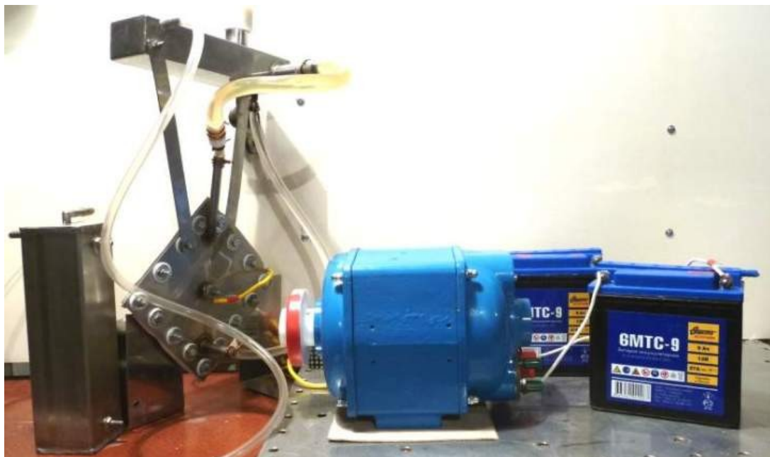
Fig. 6. Photo MG-2 + 2 accumulators 6MTC-9 + a cell of electrolyser
