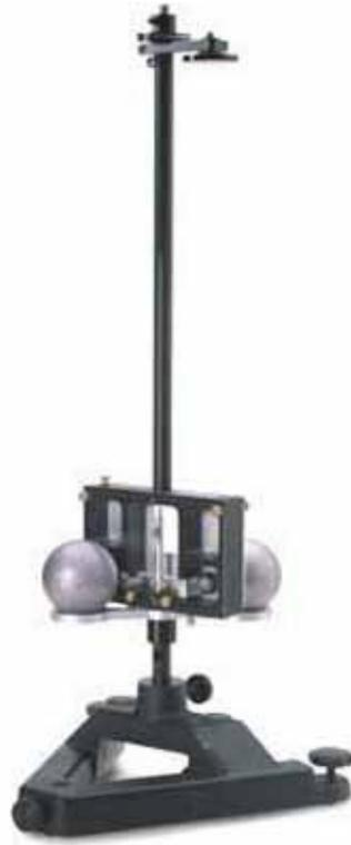
I would estimate these large lead balls to be 3 inches, at the most. Pasco tells us they are 3.3lbs, about twice the weight of Cavendish's small balls. In the next one we see even smaller balls.
