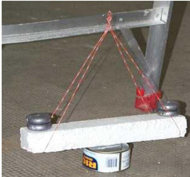
The small mass is a lead fishing weight, weighing only an ounce or so. The large weights are not pictured, but they are steel spheres about three inches in diameter. This last guy, John Walker of Fourmilab (not to be confused with Fermilab), tells us to make sure to put the apparatus away from the walls, which he has found may skew the findings. This is the only good advice in an otherwise terrible experiment. Despite this it is reproduced all over the internet, sold as a thing of beauty.
