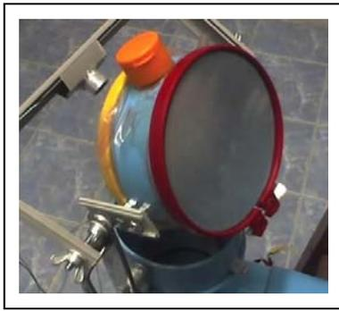
Each acoustic plate is therefore like a 50 mm thick disk, or drum, having two parallel surfaces of thin elastic membranes that separate the interior of the plate from the exterior (left picture).
