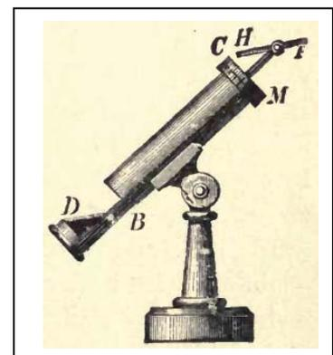
The angle between the planes of reflection of the two glass plates can be changed by rotating the second glass plate around the beam of light reflected by the first.
