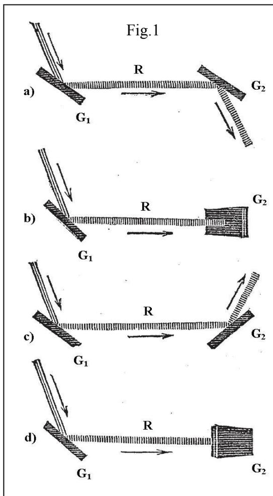
This behavior of the beam of light (R) is quite remarkable because normally beams of light reflect from glass plates no matter on which side of the beam the glass plate is and irrespective of the angle of incidence. Still, in this case, the light beam (R) reflects or not from the second glass plate (G<sub>2</sub>), depending on the side of the beam on which the glass plate is placed for reflection and on whether the angle of incidence is different from or equal to 56 degrees.
