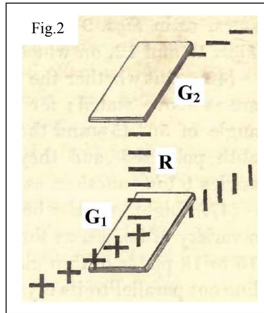
Then, following the same logic consistently, it was argued that, upon incidence on the second glass plate ( $G_2$ ), reflection will take place according to whether the glass surface was parallel or not to the oscillations composing the beam of light (R). (Fig.2 is reproduced and adapted from [4]).
