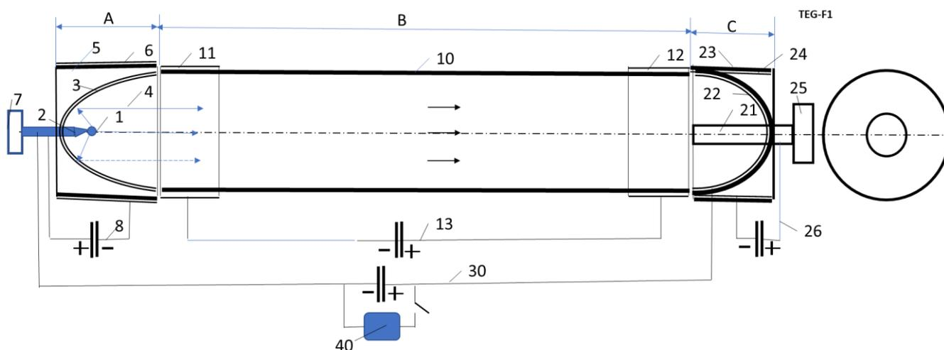
Fig.2. Cylindrical Impulse thermonuclear electric generator. *Nomenclature*: Section A (thermonuclear micro-reactor and collector of negative particles-electrons): 1 - micro-fuel capsule, 2 – deliver of fuel capsule and electric energy, 3 – electrostatic mirror, 4 – trajectories of nuclear, 5 – positive electrode of the electron collector, 6 – isolator, 7 – issue of ignition and mechanism for delivery of fuel; section B (brake of nuclear): 10 – isolation pipe, 11-12 brake
