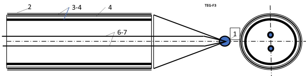
Fig. 4. Deliver of fuel capsule and electric energy for Fig.2-3. *Nomenclature:* 1 - fuel capsule, 2 - conductive layer, 3-4 – isolator, 4 - conductive layer, 6-7 – delivery energy (electricity) to fuel capsule.
