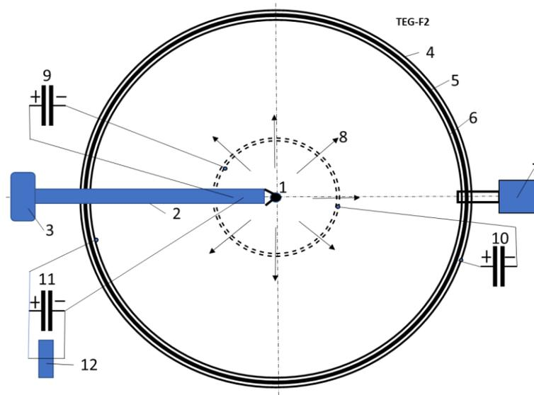
Fig.3. Spherical Impulse thermonuclear electric generator. *Nomenclature:* 1 - micro-fuel capsule, 2 – deliver of fuel capsule and electric energy, 3 – issue of ignition and mechanism for delivery of fuel, 4 – outer electrode of brake, 5 – isolator, 6 – inter (positive) electrode of collector, 7 – vacuum pump, 8 – trajectory of nuclear.
