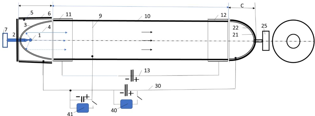
Fig.1. The simplest cylindrical Impulse thermonuclear electric generator. *Nomenclature:* Section A (thermonuclear micro-reactor and collector of negative particles-electrons): 1 - micro-fuel capsule, 2 – deliver of fuel capsule and electric energy, 3 – three net electrostatic mirror, 4 – trajectory of positive nuclear, 5 – electrode of the electron
