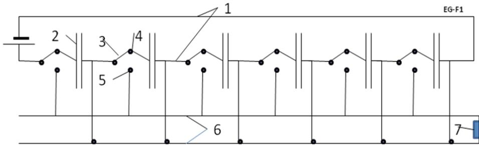
Fig.2. Principal Schema of the offered transformer -- high voltage DC in low voltage DC or DC in AC and back. *Notations:* 1 – high voltage line, 2 – condensers (capacitor), 3 – two positions electronic switch, 4 – contact the high voltage line, 5 – contact the low voltage line, 6 – low voltage line. 7 - outer electric load.
