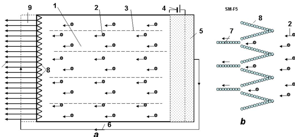
Fig. 10. Method particle traps for production of the AB-needles. *Notations:* a – device; b – particle traps; 1 - vacuum cell; 2- charged particles; 3 – magnetic lines; 4 – electric issue for the acceleration nets; 5 - plasma from particles; 6 – flow of electrons; 7 – AB-needles; 8 – trap made from AB-matter for the charged particles ( $p$ ,  $^2\text{H}$ ,  $^4\text{He}$ , etc.); 9 – cell for cover the AB-needles by electrons.
