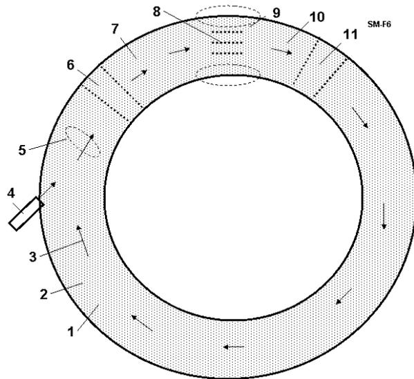
Fig. 9 Toroid producer of AB-needles (AB-matter). *Notations:* 1 – vacuum toroid; 2 – perpendicular (to sketch) magnetic lines; 3 – particles; 4 - particles gun; 5 – round magnetic lines from motion charged particles; 6 – electric accelerator; 7 – electric focuser; 8 – AB – needles; 9 – magnetic field keeping the AB-needles; 10 – electric focuser; 11 – electric accelerator.
