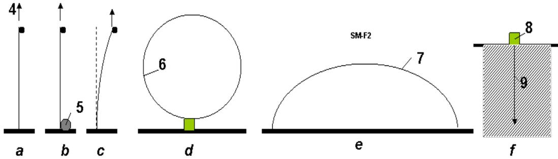
Fig. 6. Some construction from AB-string. *Notations:* *a* – vertical string (AB-needle). The big lift (support) force *4* does not depend from length; *b* – lifting the load to any altitude. *5* – spool of AB-string; *c* – stability of AB-string; *d* – ring *6* from AB-string; *e* – bridge (long arm) from AB-string; *f* – research of the Earth crust interior: *8* – installation (spool of AB-needle), *9* – AB-needle (string, cable).
