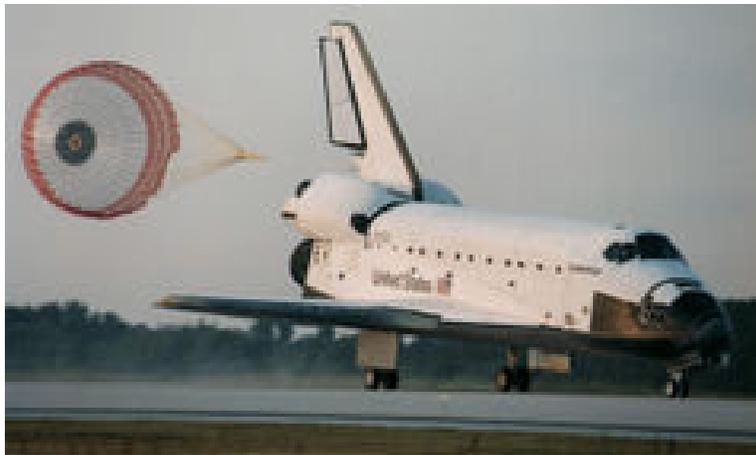
**Fig. 8** . Endeavour deploys drag chute after touch-down the Shuttle.(Credit NASA)
