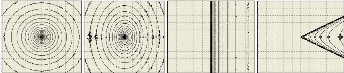
Figure 1: Logarithm of the retarded potential of uniformly moving charge ( $v=0, v<c, v=c, v>c$ ) with its current position in origin  $[0,0]$  (the centre of each chart). The charge of particle does not vary in time.
