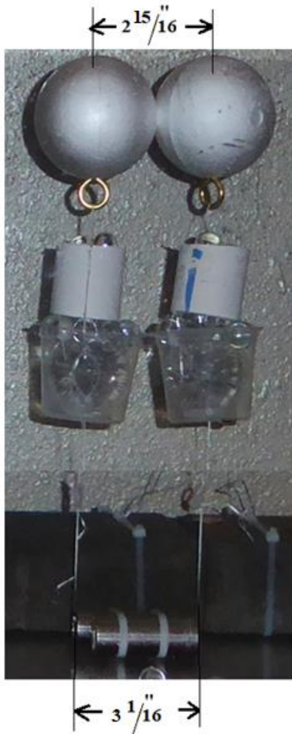
Fig 4 A Closer-up View of the Two Floating Balls (The Strings between the Socket and the Cups in This Picture Are Shortened via Computer Effect for a Better View)
