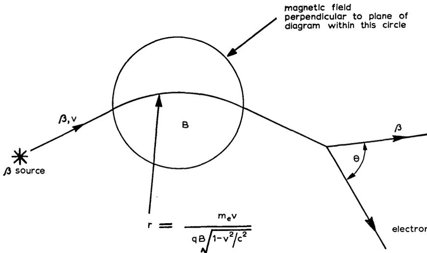
1 Champion's experiment on the collision of fast  $\beta$  particles with an electron. The particles' velocities are calculated from the curvature of their paths in the magnetic field  $B$
