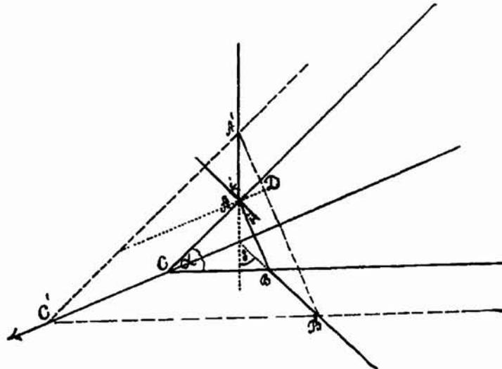
Suppose that the ray passes through the prism at the angle of minimum deviation, which we shall denote by  $\delta$ . The prism is moving in the direction of  $CC_1$  at the rate  $c$ , and its side faces are supposed to be unlimited in their length.
