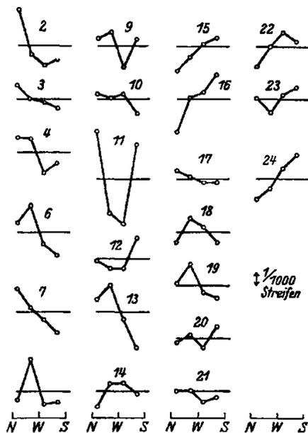
Strip shifts with the turn of the apparatus. (The written down directions refer to the direction of the emphasized arm)
