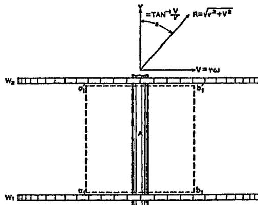
FIG. 1. Plan view of double Fizeau toothed wheel.
