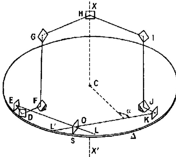
rotation of the disc. For all the mirrors other than  $F, G, I, J$ , the planes of incidence are horizontal, parallel to the disc. Only the planes of incidence of the mirrors  $F, G, I, J$  are vertical and contain the axis of rotation  $XCX'$ . These mirrors are tilted with  $45^\circ$  on the vertical,  $F$  being parallel with  $G$ , and  $J$  parallel with  $I$  at the time of the flash, carried out here in white light.  $FG$
