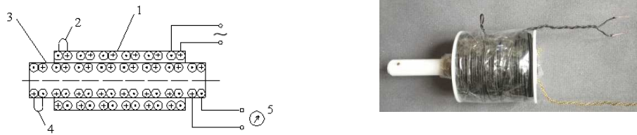
Fig. 6. Electromagnetic induction between two solenoids with zero magnetic field. 1. Primary coils, 2 place of bending, 3 secondary coils, 4 place of bending, 5 voltmeter
