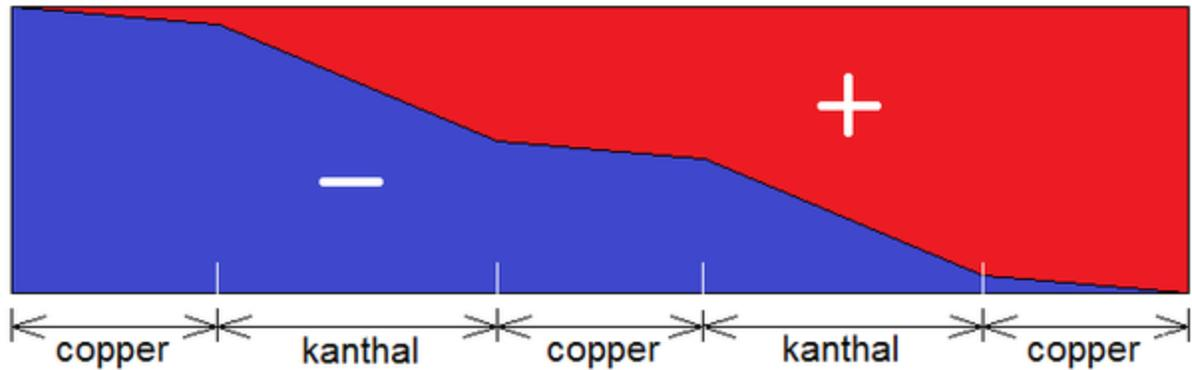
Two pieces of a highly resistive alloy (Kanthal) and three pieces of copper wire are connected in series. The two kanthal pieces are actually two resistors. We see that the ratio Plus/Minus along the kanthal sections changes much more rapidly than along the copper sections. The middle copper section corresponds to the neutral wire.
