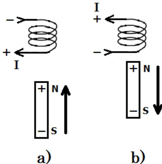
When we move the magnet toward the coil, then the induced current in it has such a magnetic field that it resists the movement of the magnet, that is, it repels the magnet. When we move the magnet away from the coil, then the induced current in it has such a magnetic field that it resists the movement of the magnet again, that is, it attracts the magnet (this is the so-called Lenz's law).
