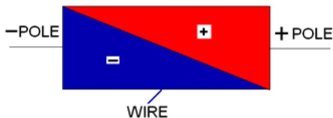
Let's say the DC source is of a pretty high voltage. If we touch with one hand one of its terminals and with the other hand a large electrically conductive object (which is not otherwise connected with the circuit), then we can sense an electric shock. However, if we do the same again, but this time touching **the middle of the connecting wire**, then nothing will happen, that is, we won't sense anything. Why?
