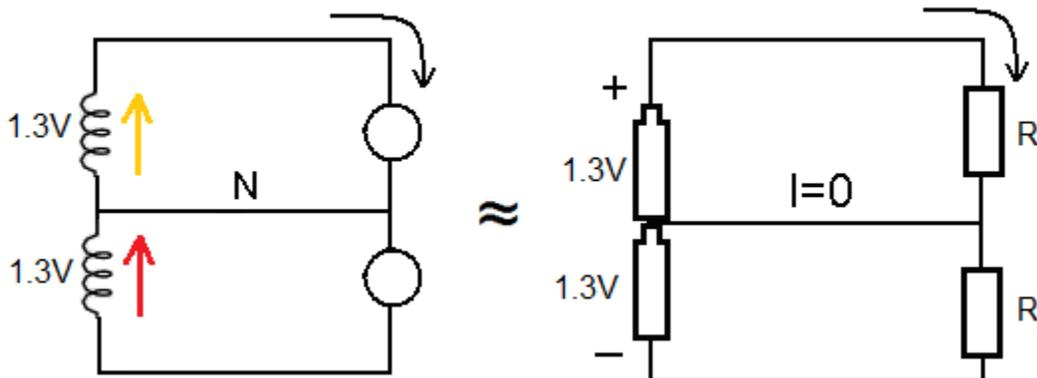
Let's consider now the moment marked with No.2. The current in the red coil has risen to the positive maximum, whereas the current in both other coils is exactly half of the negative maximum. The situation in this moment can figuratively be represented in the following way:
