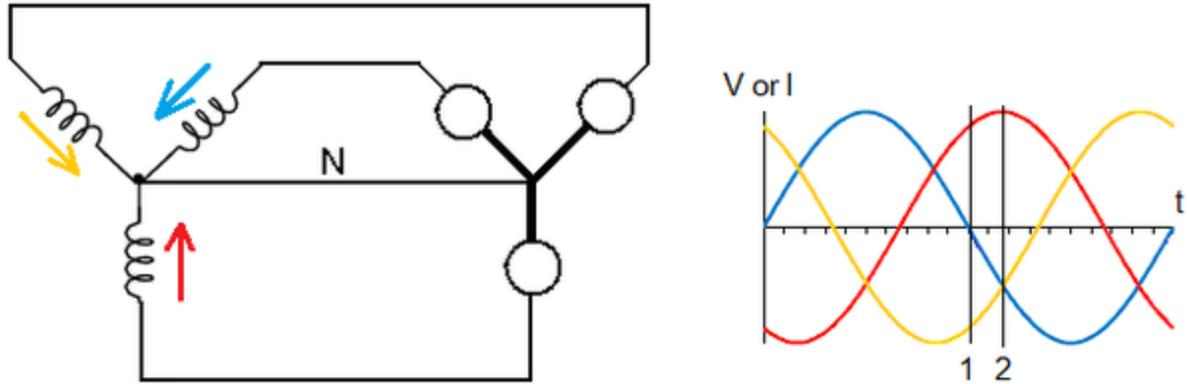
On the left side is shown a three phase generator with **three identical lamps** connected to it - one lamp to each phase (**so-called balanced load**). The coils as well as the lamps are in star-connection. The central points of the stars are connected with a wire. It is the neutral wire.
