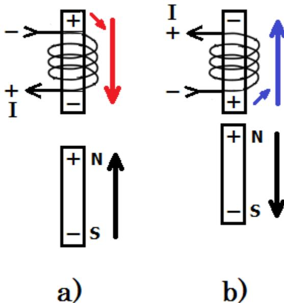
But inducing a current in a coil by oscillatory motion of a magnet is not feasible in practice. Therefore, the current in the generators is induced by rotational motion of a magnet. Look at figure below:
