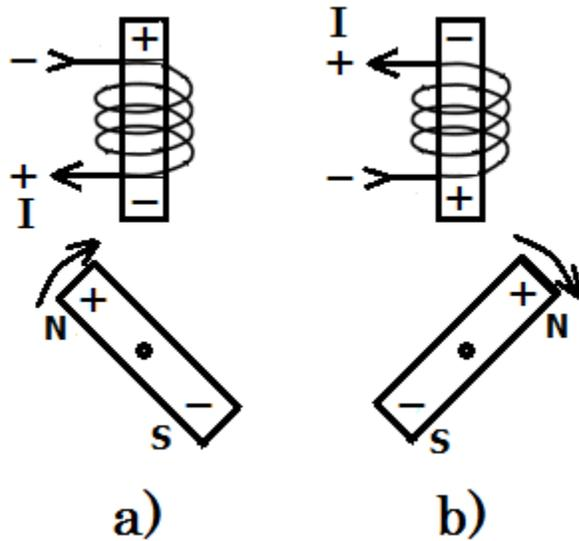
The magnet, which sits on the same axle as the turbine, is rotating clockwise. When the Plus-pole is approaching the coil with the iron core (figure **a**), then it is comparable to the situation **(a)** of the second to last figure. When the Plus-pole is moving away from the coil with the iron core (figure **b**), then it is comparable to the situation **(b)** of the same figure. When the magnet is, so to say, face to face with the coil, then the induced current drops to zero.
