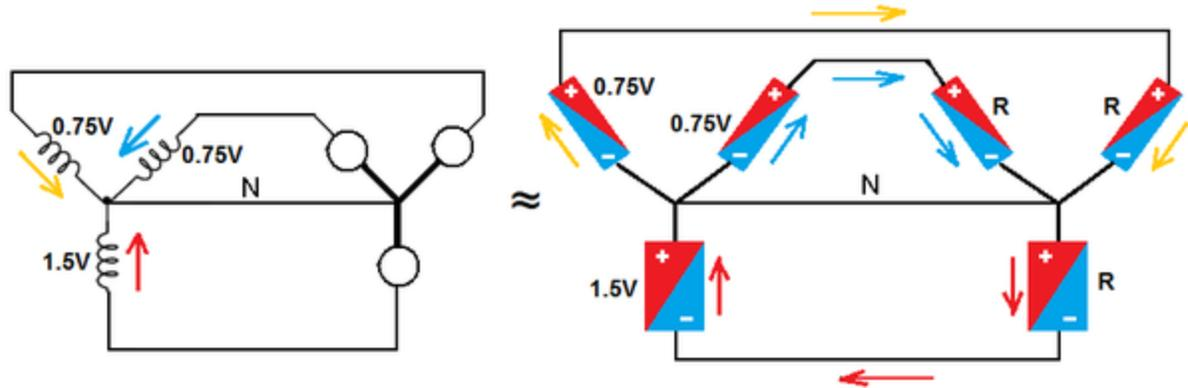
Look please at the figure on the right. With the colored arrows are now shown **the factual directions** of the currents through the branches. As we can see, the blowing of the red coil toward the star-point is ideally met by two equal suctions of the other coils. The same applies also to the star-point on the resistor's side, only the directions are reversed.
