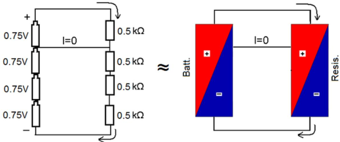
What has just been said does not apply only between generator's and load's side, but also between resistors connected in parallel. Look please at the figure below:
