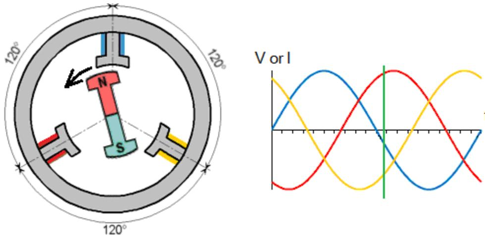
The magnet in the diagram is turning counter-clockwise. With the vertical green line in the graph on the right is marked the moment, that is, the position of the magnet in the left diagram. The faster the magnet is turning, the greater will be the frequency as well as the induced voltage/current.
