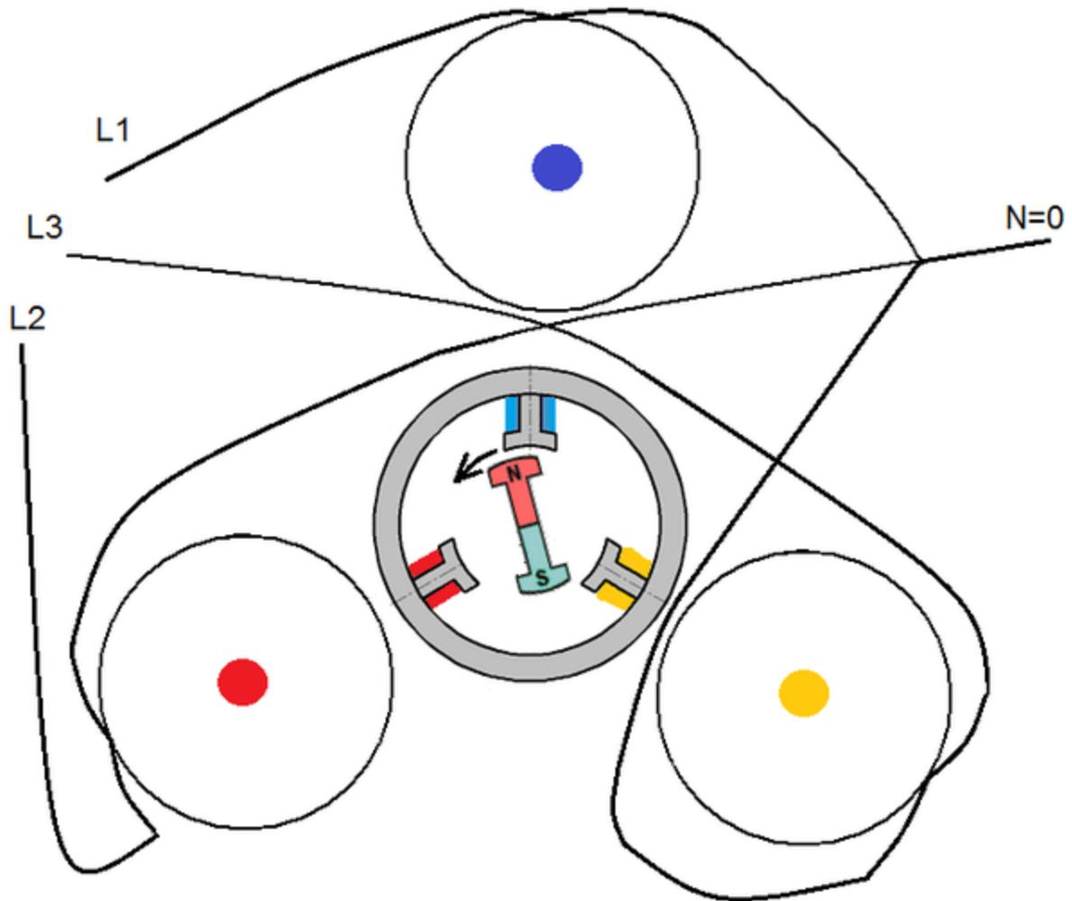
When the North-pole of the magnet is moving toward the red coil, then the left end of the coil will be Plus and the right end will be Minus. The same will happen when the North-pole is moving toward the other coils. Only in this way we will get a proper arrangement of the sine curves and consequently a proper Neutral.
