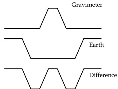
Fig. 2. The shielding effect on the Earth is registered as negative by the gravimeter. The registration contains therefore the difference between effect on the gravimeter and effect on the Earth.
