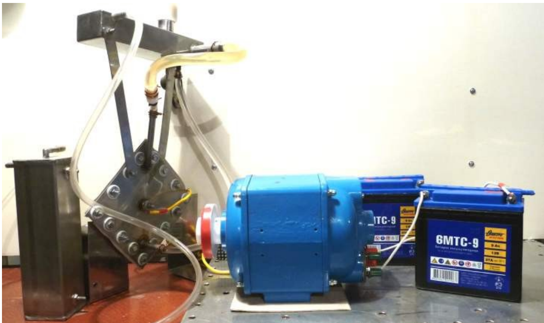
Fig. 4. Photo of MG-2 +2 6MTC-9 accumulators + the electrolyser cell
