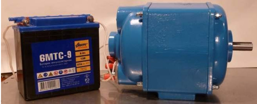
Fig. 3. MG-2 motor-generator and the motorcycle accumulator for its supply
