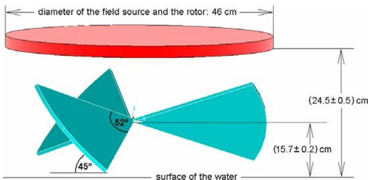
FIG. 4. Principle design of an electrostatic rotor for the conversion of vacuum-energy into mechanical energy. The disc (red) is electrically charged, whereas the rotor (blue) is connected to ground. The specified dimensions represent the values in the setup of the experiment described.
