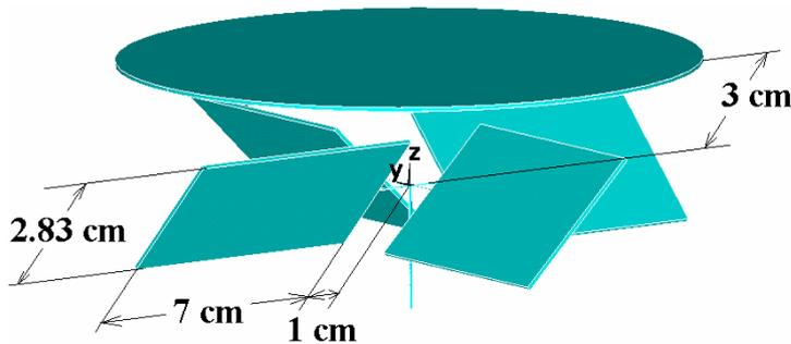
FIG. 8. Visualization of a superconducting rotor, which is mounted on an axis below a flat permanent magnet. The dimensions will be used for a numerical example.
