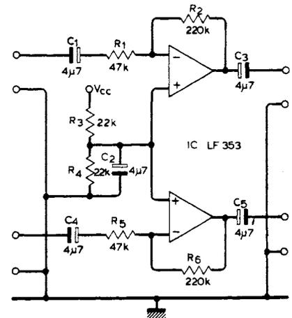
Circuit for 60dB display range, left, uses LW3915  $V_{cc}$  24V,  $V_{gg}$  12V. Buffer circuit, above, and board patterns are for use with medium-impedance outputs.  $V_{cc}$  can be 15 to 30V, unregulated. In the p.c.b. pattern on page 32 (August issue), pins b & 1 of IC3 should be linked to pins 4 & 8 of IC4.
