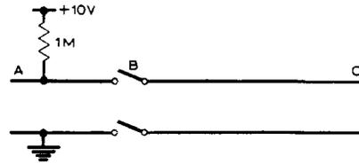
A five-volt pulse two metres wide was found to travel off to the right at the speed of light for the dielectric on closure of the switches, leaving the section AB completely discharged. (The practical device lacked the second, lower switch at B, which is added in the diagram to simplify the argument).
