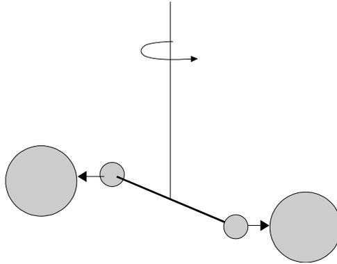
Torsion balance for measuring molecular forces between macroscopic bodies. Weak forces are magnified by using as much matter as possible concentrated in two or four spheres, and then measuring torsion of the wire which holds smaller weights.
